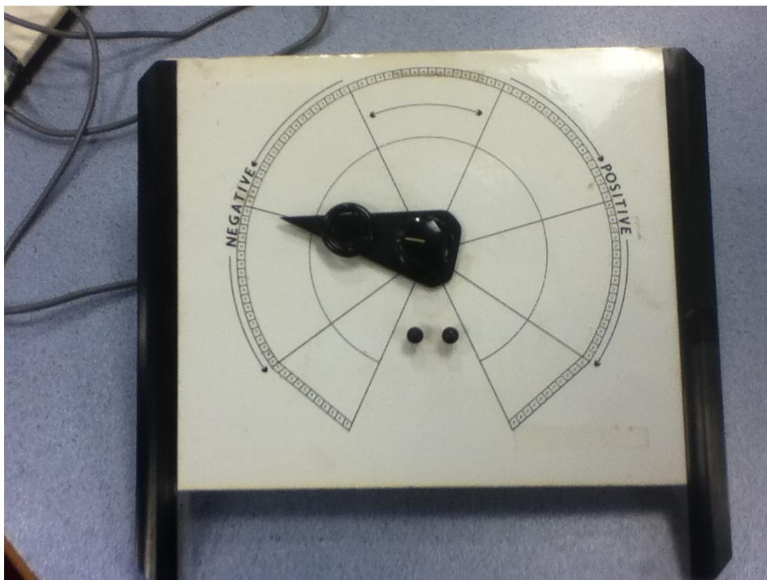
**Figure 2.1.** The dial version of the Continuous Response Digital Interface (CRDI).
